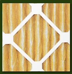
final or prefilter. MERV 11 rated filters must average between 65% and 80% minimum removal efficiencies on the four particle size ranges from 1 to 3 microns in size per ASHRAE 52.2. This particle size range is specifically a target because it represents the size of most airborne biological matter.
