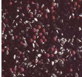
Carbon, Impregnated Alumina and Zeolite Blend
