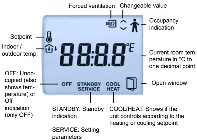
It is possible to set different parameter values in a parameter menu in the display, using the buttons on the controller. You change parameter values with the INCREASE and DECREASE buttons and confirm changes with the Occupancy button.
